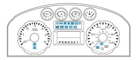
Warning lights and gauges can alert you to a vehicle condition that may become serious enough to cause expensive repairs. A warning light may illuminate when a problem exists with one of your vehicle's functions. Many lights will illuminate when you start your vehicle to make sure the
